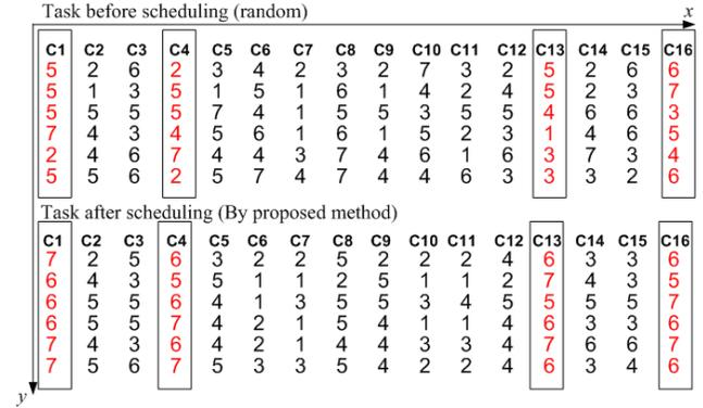
Fig. 7. Task assignments on different cores before (random) and after the proposed scheduling method. Boxed columns are tasks executed on corner cores. The larger task id represents heavier task.
