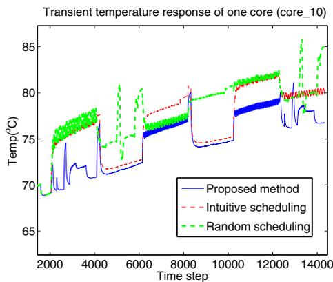
Fig. 10. Comparison of transient temperature responses using different task scheduling schemes
