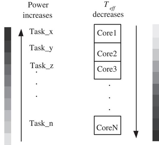
Fig. 3. Proposed new task assignment scheme based on  $T_{eff}$
