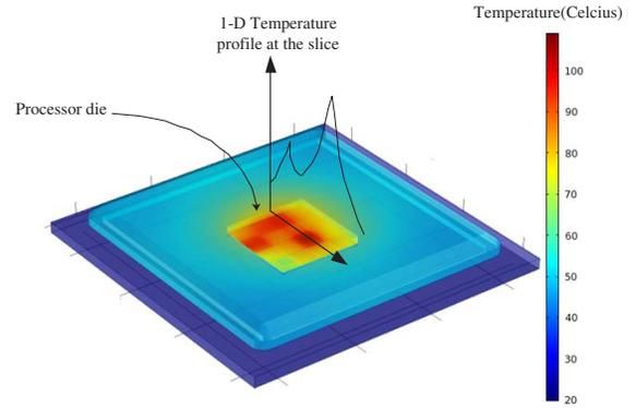
Fig. 1. Temperature profile of a multi-core microprocessor package
