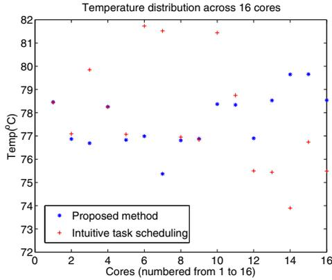
Fig. 9. Temperature distribution across the cores (time step 11600)
