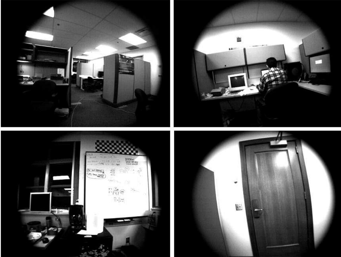
Figure 2: Some example images from the sequence recorded during the indoor experiment. Note the severe distortion caused by the use of a 4mm-lens with a relatively wide field of view (55 degrees). This lens also causes the image to be projected in the central part of the CCD sensor, resulting in "blacked-out" areas in outer parts of the images.
