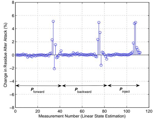
Fig. 4. Changes in the residue corresponding to each measurement after implementing a *nonlinear* FDIA against *linear* state estimation.
