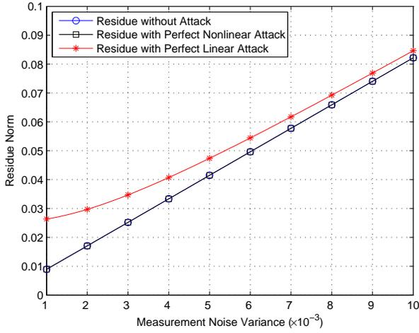
Fig. 6. Residue vs. measurement noise for perfect nonlinear FDIA.
