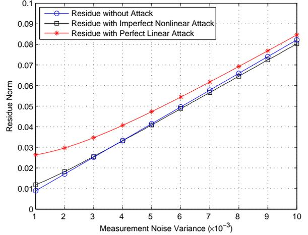
Fig. 7. Residue vs. measurement noise for imperfect nonlinear FDIAs.
