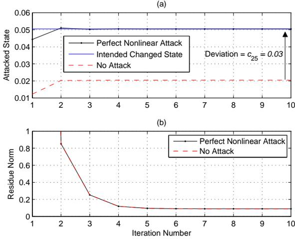
Fig. 2. Performance of a perfect nonlinear FDIA over iterations of nonlinear state estimation: (a) State estimation solution. (b) Residue norm.
