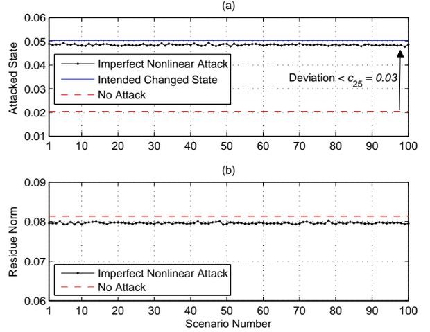
Fig. 3. Performance of an imperfect nonlinear FDIA for 100 different attack inaccuracy scenarios: (a) State estimation solution. (b) Residue norm.
