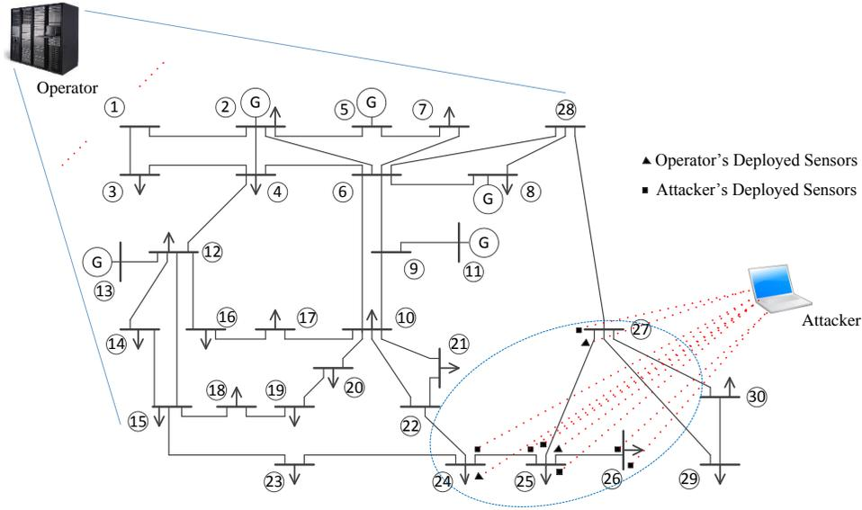
Fig. 1. State estimation in an IEEE 30 bus system. The attacker collects local information to implement an FDIA attack against the phase angle at bus 25.
