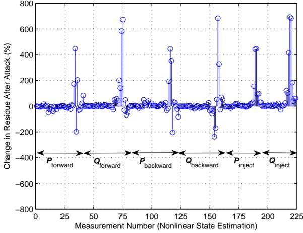
Fig. 5. Changes in the residue corresponding to each measurement after implementing a linear FDIA against nonlinear state estimation.
