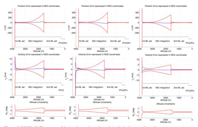
Figure 9. VISINAV filter errors (blue) and covariance bounds (red) during parachute descent.
