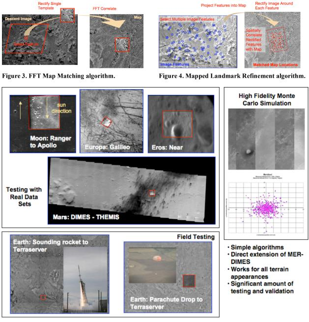
Figure 5. Data sets used for testing the mapped landmark matching algorithm.
