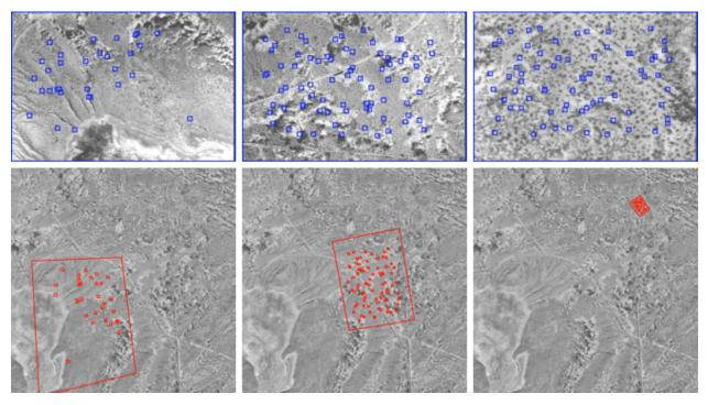
Figure 6. Mapped landmark matches between the map (red) and the descent image (blue) for three altitudes (left is 1600 m AGL, middle is 900 m AGL, right is 230 m AGL).
