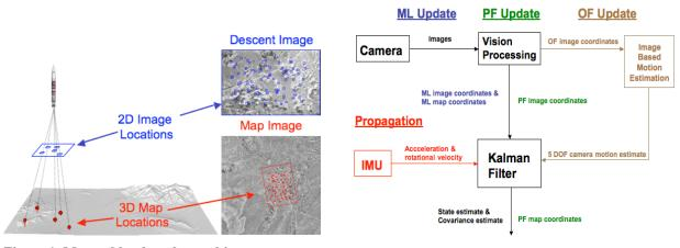
Figure 1. Mapped landmark matching concept.
